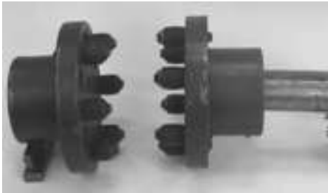
Figure 3.7 - A type of direct coupling
